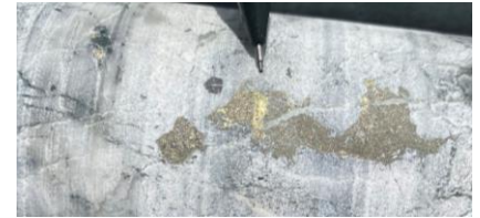
BBDD014 (above) and BBDD020 (below): Visible gold within pyrite in c.20cm wide quartz-tourmaline veins at 72.50m and 69.50m downhole respectively
