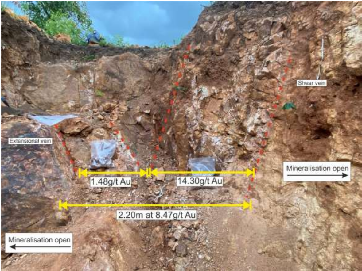
Figure 9. MBTR001 (viewing towards the South) showing approximate location of sampling over intersecting shear and extensional quartz vein sets.
