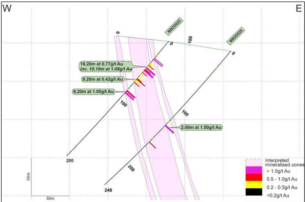
Figure 31. Simplified cross section for fence line N874133, viewing N-S and showing the results of MBDD038 drilled towards the south, and where it intersects fence line N874091
