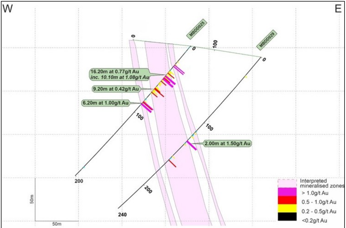
Figure 33. Simplified cross section for fence line N874318 with results from MBDD025 and MBDD029 and interpreted mineralised zones.
